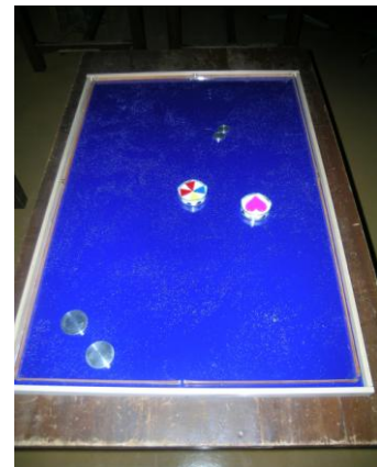
Figure 3 (a) big frictionless glass plate equipped with a large-angle-frictionless slope (a) (b) Small frictionless glass plate.
